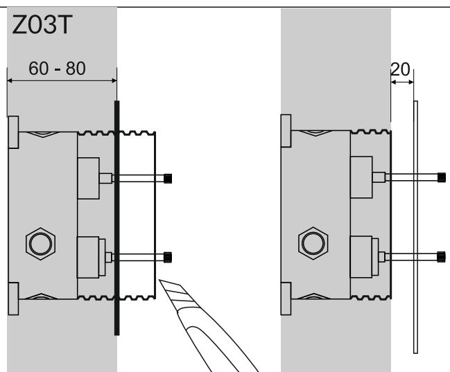
Correctly installed box should be placed at a depth that takes into account the thickness of the ceramic tiles and glue. The depth is set individually.
