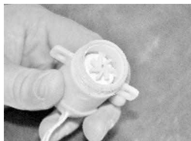
5. Hydro generator's turbine
