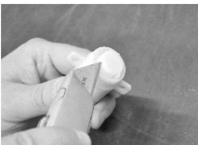
4. Taking out the turbine protection
